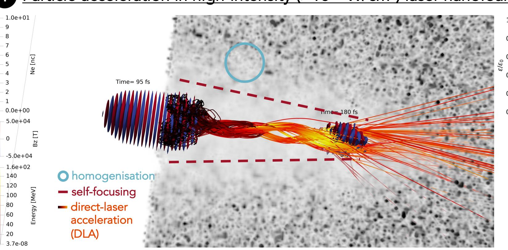
Strongly magnetised plasma channel driving electron betatron oscillation. High energy spectrum tail due to direct laser acceleration.
