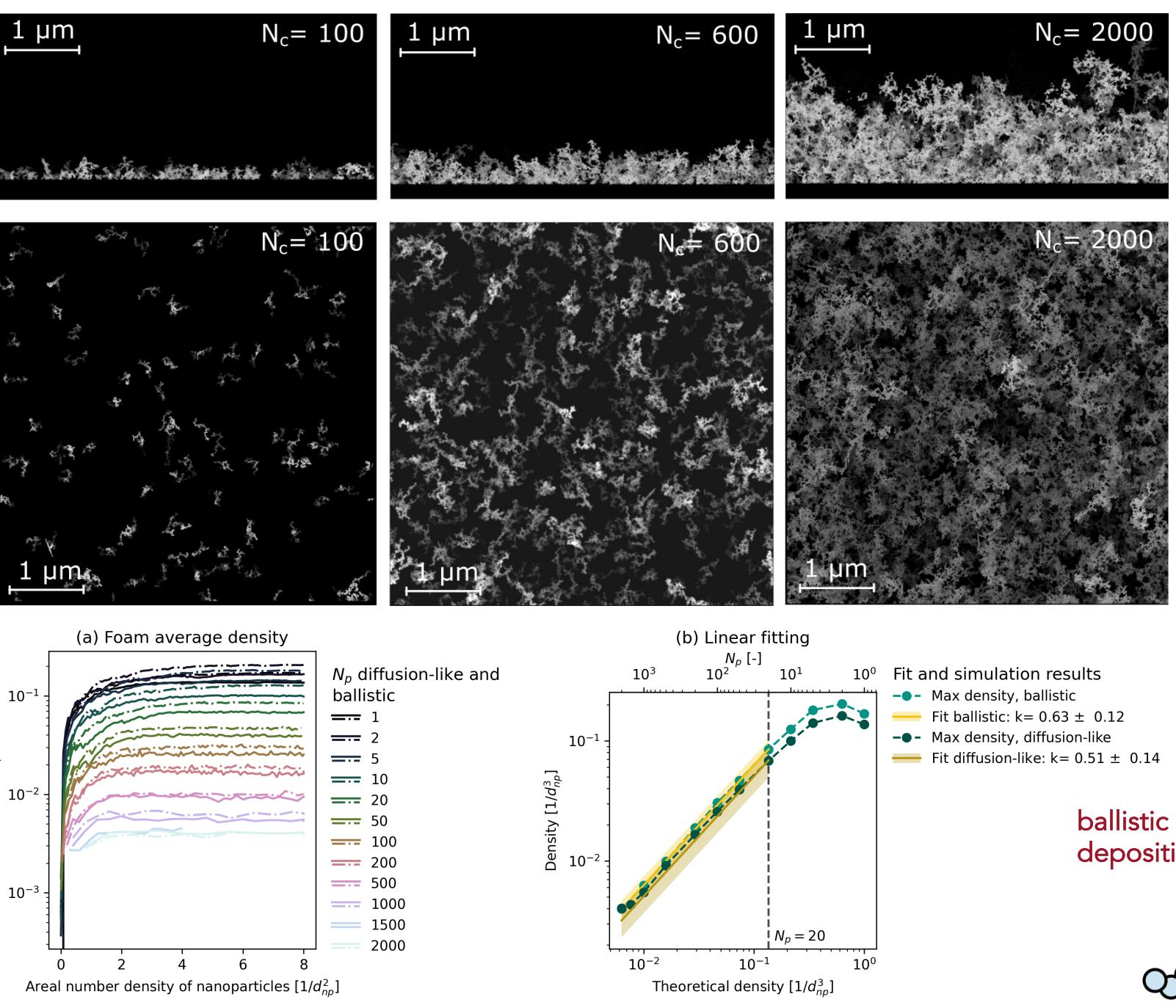
Low-density nanofoams are fractal materials. Their density related to the component dimension ( $R_g$ ) with fractal scaling with number of particles per cluster ( $N_p$ ):
