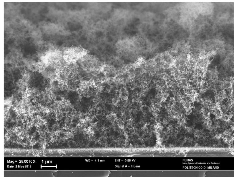
Produced with Pulsed Laser Deposition (PLD)
