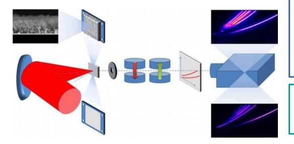
Up to 5x10<sup>20</sup> W/cm<sup>2</sup> 30 fs, 30° pulse incidence C-,P-,S- polarization
